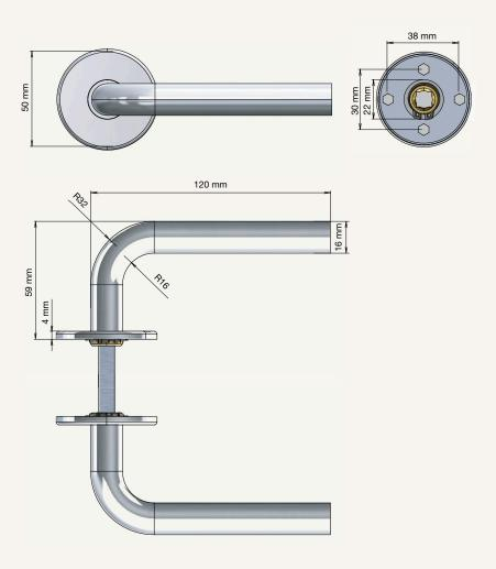
MATERIAL: STAINLESS STEEL AISI 304 AVAILABLE IN TWO FROST FINISHES:
