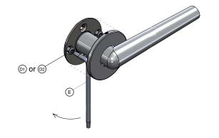
Secure the handle on the spindle  $\widehat{\mathbb{A}},$  by using the hex key  $\widehat{\mathbb{F}}$  to tighten the set screw.
