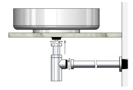
To empty and clean the bottle trap, use a coin or a suitable tool to loosen the bottom cap ①, and empty out the water and any remaining waste.
