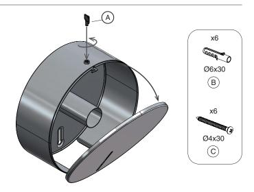
Place the dispenser in the desired position and mark the screw holes as illustrated.
