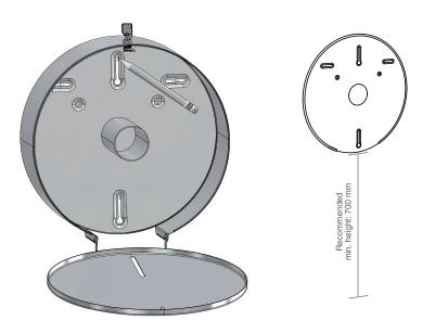
Drill the marked holes using a 6 mm drill bit and insert the enclosed Ø6x30 mm wall plugs (B).
