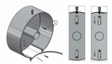
Use the remaining 4 4x30 mm screws © to fully secure the toilet roll holder to the wall.
