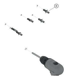
Use 2 of the enclosed 4x30 mm screws © to secure the toilet roll holder to the wall using a PH2 bit.
