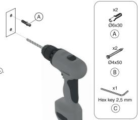
Secure the brass inserts on the wall with the enclosed Ø4x50 mm screws (a) and use a Phillips screwdriver with bit PH2 to tighten the screws.
