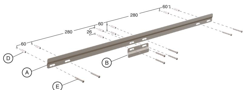
Slide the shelf (C) onto the mounting bracket (A) and (B).
