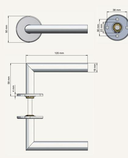
MATERIAL: STAINLESS STEEL AISI 304 AVAILABLE IN TWO FROST FINISHES:
