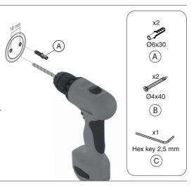
Secure the insert on the wall with the enclosed Ø4x40 mm screws (B) and use a Phillips screwdriver with bit PH2 to tighten the screws.
