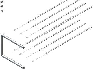
Mount the opposite side frame © onto the ends of the eight crossbars (B). This may also require small rotational movements.
