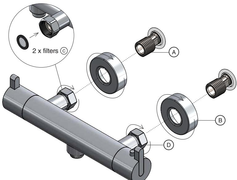
8 Remove the red and blue caps on the mixer and insert the two Filters **C** into the inlets of the thermostatic mixer as illustrated.
