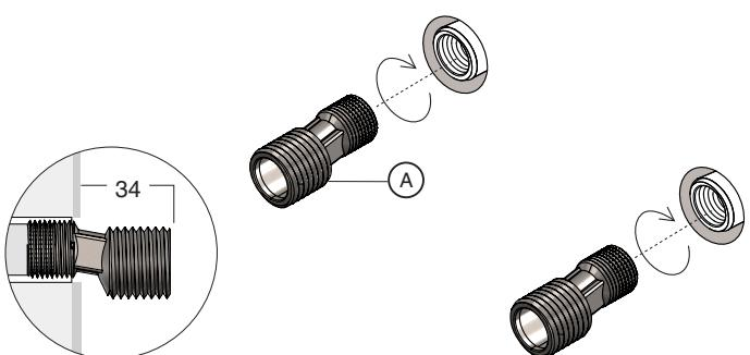
4 When in the right positions make markings, and then remove the connections.
