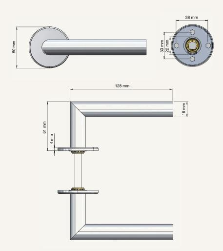
MATERIAL: STAINLESS STEEL AISI 304 AVAILABLE IN TWO FROST FINISHES:
