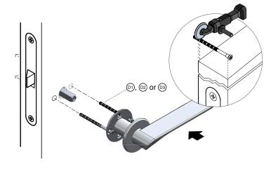
Use the enclosed torx key no. 15  $\stackrel{\frown}{\mathbb{E}}$  to tighten the machine screw  $\stackrel{\frown}{\mathbb{D}}$  or  $\stackrel{\frown}{\mathbb{D}}$  until fastened.
