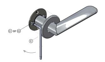
Secure the handle on the spindle  $\widehat{\mathbb{A}},$  by using the hex key  $\widehat{\mathbb{F}}$  to tighten the set screw.
