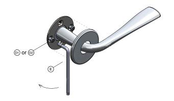
Secure the handle on the spindle  $\widehat{\mathbb{A}},$  by using the hex key  $\widehat{\mathbb{F}}$  to tighten the set screw.
