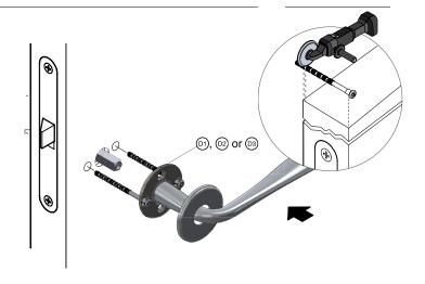
Use the enclosed torx key no. 15  $\stackrel{\frown}{\mathbb{E}}$  to tighten the machine screw  $\stackrel{\frown}{\mathbb{D}}$  or  $\stackrel{\frown}{\mathbb{D}}$  until fastened.
