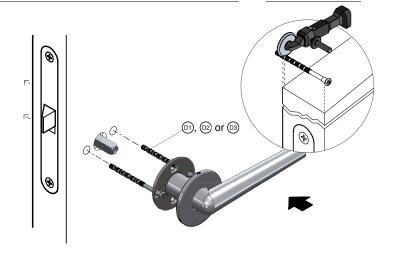
Use the enclosed torx key no. 15  $\stackrel{\frown}{\mathbb{E}}$  to tighten the machine screw  $\stackrel{\frown}{\mathbb{D}}$  or  $\stackrel{\frown}{\mathbb{D}}$  until fastened.
