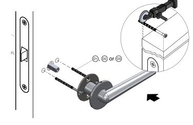
Use the enclosed torx key no. 15 (E) to tighten the machine screw (1) or (2) until fastened.
