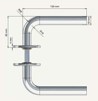
MATERIAL: STAINLESS STEEL AISI 304 AVAILABLE IN TWO FROST FINISHES:
