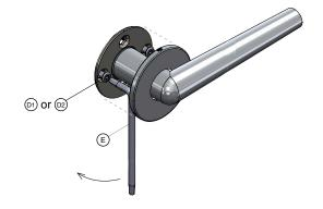
Secure the handle on the spindle (A), by using the hex key (F) to tighten the set screw.
