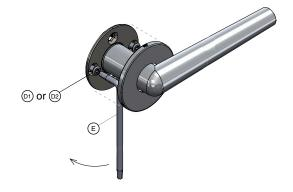
Secure the handle on the spindle (A), by using the hex key (F) to tighten the set screw.
