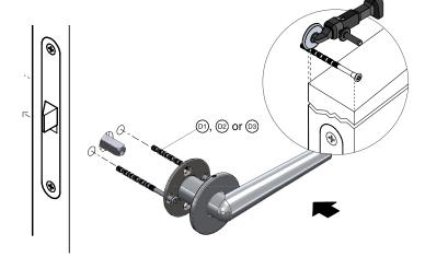
Use the enclosed torx key no. 15 (E) to tighten the machine screw (D) or (D) until fastened.
