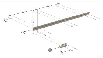
Slide the shelf © onto the mounting bracket A and B.
