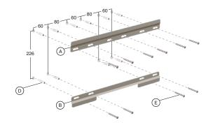
Slide the shelf c onto the mounting bracket A and B.
