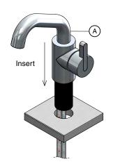
Slide the NBR washer  $\bigcirc$  and stainless steel washer  $\bigcirc$  onto the threaded sleeve B, then screw on the fixing nut E while holding the tap in place.
