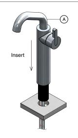
Slide the NBR washer  $\bigcirc$  and stainless steel washer  $\bigcirc$  onto the threaded sleeve B, then screw on the fixing nut E while holding the tap in place.
