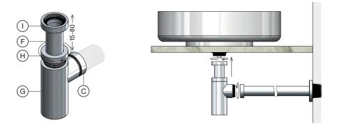
To empty and clean the bottle trap, use a coin or a suitable tool to loosen the bottom cap (J), and empty out the water and any remaining waste.
