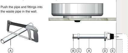
To connect the inlet pipe  $\bigcirc$  and the bottle trap  $\bigcirc$  to the setup, start by screwing the fitting nut  $\bigcirc$  onto the bottle trap.
