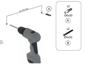
Secure the Clamp on the wall with the enclosed Ø4x30 mm screws ® and use a Phillips screwdriver with bit PH2 to tighten the screws.
