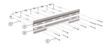
Slide the shelf © onto the mounting bracket (A) and (B).
