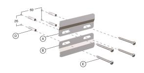
Slide the shelf  $\bigcirc$  onto the mounting bracket  $\bigcirc$  and  $\bigcirc$  .
