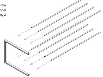
Mount the opposite side frame ⓒ onto the ends of the eight crossbars (B). This may also require small rotational movements.
