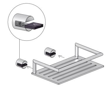
Securely tighten the set screws D located underneath the brackets with the hex key C, ensuring the shelf is firmly fixed.
