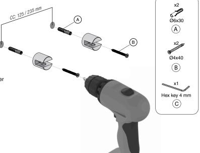
Place the rubber spacers inside the brackets.
