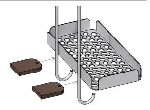
To attach the Shower Shelf to the shower mixer, gently squeeze the two metal hooks together and slide them up between the mixer valves.
