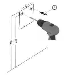
Secure the Seat on the wall with the enclosed M10x90 mm screws (a) and two ø16 mm lock washers (c). Use a 8 mm hex key (d) or hex bit to tighten the screws.
