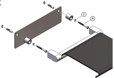
Tighten the bolts underneath the Seat on each side with the 4 mm hex key  $\bigcirc$ .
