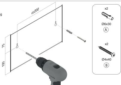
Lift the dispenser onto the screws and slide it down until it locks into place. Gently tighten the screws to ensure the dispenser is securely mounted.
