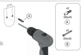
To secure the Dispenser Holder on to the wall, first put the bushings ©, and then the threaded washers © onto the enclosed Ø4x30 mm screws (B).
