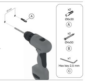
Secure the insert on the wall with the enclosed Ø4x50 mm screws (B) and use a Phillips screwdriver with bit PH2 to tighten the screws.
