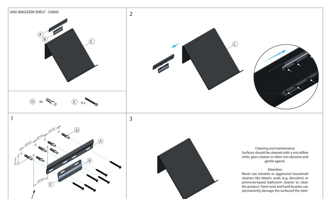
The lower bracket should only be mounted if the shelf is installed in a public area with risk of people removing the shelf.
