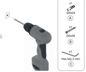
Secure the Camouflage foot on the wall with the enclosed Ø3x28 mm screw (B) and use a Phillips screwdriver with bit PH2 to tighten the screw.
